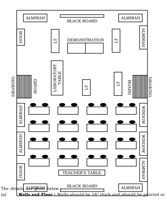
distempered. Floor should be perfectly smooth with cement plaster. Round corners between the wall and floors are recommended.
