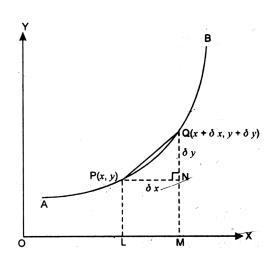
Similarly the resolved part of the velocity parallel to OY =  $\underset{\delta t \to 0}{\text{Lt}} \frac{\delta y}{\delta t} = \frac{dy}{dt}$ If V is the resultant velocity making an angle  $\theta$  with OX, then
