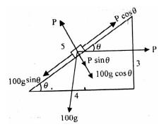
(i) Its weight 100g N acting vertically downwards. It can be resolved into two components 100g sin  $\theta$  down the plane and 100g cos  $\theta$  perpendicular to the plane.
