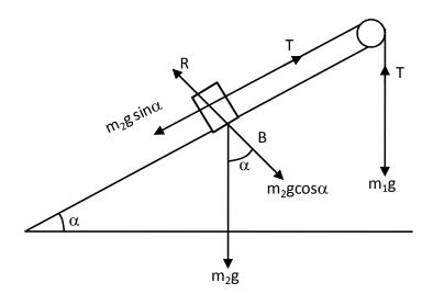
(i) its weight  $m_2 g$  acting vertically downwards which has got components  $m_2 g \sin \alpha$  down the plane and  $m_2 g \cos \alpha$  perpendicular to the plane.
