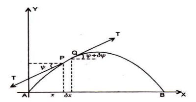
PQ of the string between its points P (x, y) and Q  $(x + \delta x, y + \delta y)$ , where the tangents make angles  $\psi$  and  $\psi + \delta \psi$  with x-axis. Clearly the element is moving upwards with the acceleration  $\partial^2 y/\partial t^2$ . Also the vertical component of the force acting on this element.
